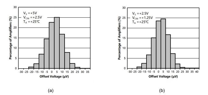
Figure 4. Offset Voltage Production Distribution at (a) +5V, (b) +2.5V
