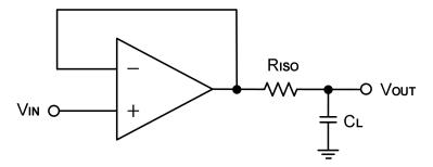
Figure 5. Indirectly Driving Heavy Capacitive Load
