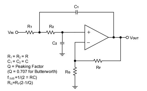
Figure 9. Two-Pole Low-Pass Sallen-Key Active Filter
