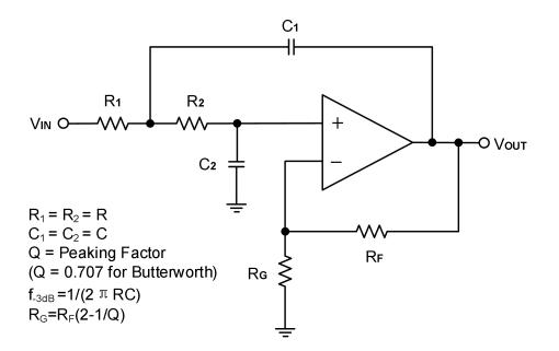
Figure 5. Two-Pole Low-Pass Sallen-Key Active Filter
