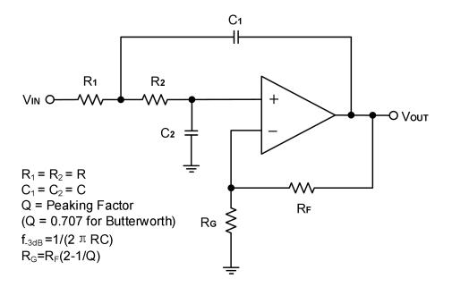
Figure 5. Two-Pole Low-Pass Sallen-Key Active Filter
